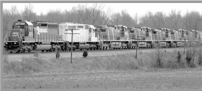
Passing through Madisonville on April 4, 2002 was this interesting lash-up. The lead unit is a CSX (ex Conrail) SD40-2, The white unit is an Alstom rebuilt SD40-2 on long term lease to CSX by CEFX. The remaining units are CEFX GE CW44ACs being returned to CEFX (a leasing company) following a short term lease to CSX.
